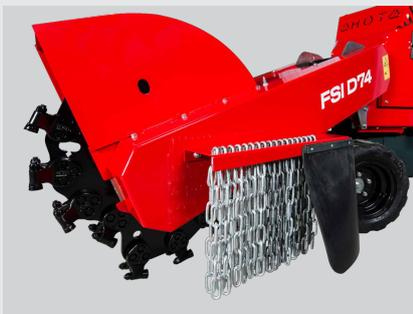
FSI D74 rapidly removes stumps thanks to its 735 mm large cutting wheel.
