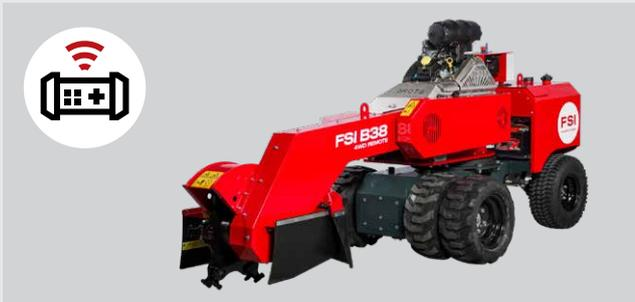
FSI B38 4WD REMOTE combines the exceptional manoeuvrability of the 4WD model with the convenience of a full-featured remote control system. This remote control allows for efficient operation while offering an excellent view of the work area. In addition, the machine is fitted a basic operating panel for ease of movement in workshops and when loading onto trailers or trucks.
