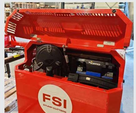
A lockable rear compartment stores the remote controller and protects the filling points from unauthorised access.
