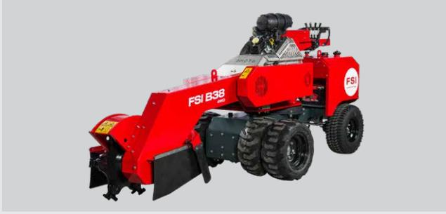
FSI B38 with 2-wheel drive offers an affordable option with all the top-tier features of the FSI B38 product family. Its swing-out operator panel and easily removable twin wheels enable a narrow 79 cm width for easy passage through garden gates. The hydraulic wheel drive with differential lock ensures traction over challenging terrain. The operator panel provides complete control of all functions, while the safety bar ensures the cutter wheel disengages upon release for enhanced operator safety.
