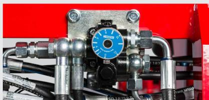
Adjust the sweep-rate to fit the hydraulic flow of your tractor and the hardness of the stump.
