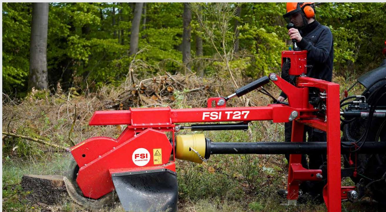
FSJ tractor-mounted stump cutters are ideal for land-clearing projects, removing stumps in orchards, municipal work in parks or along pathways and roads. Leveraging the tractor's power and all-terrain capabilities, these stump cutters efficiently remove multiple stumps in a short time, making them perfect for high-volume jobs in open-access areas.
