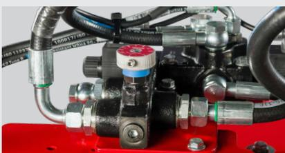
If required, the hydraulic flow rate for the sweep can be adjusted to accommodate various levels of wood hardness.
