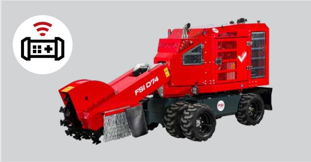
Choose between 2WD HI for long-distance travel at increased speed or 4WD LOW for enhanced traction during travel over terrain and stump cutting with FSI power-drive. Built-in hydraulic motor brakes and a counterbalance valve guarantee that the stump cutter will not slip back during grinding, providing stability and security for the operator. Storage compartments in the base frame provide convenient storage of spare parts and remote control when not in use.
