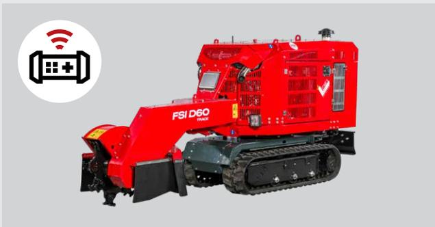
FSI D60 TRACK is equipped with counter-rotating tracks for improved manoeuvrability and superior traction in challenging terrain. Its larger contact surface evenly distributes the machine's weight, minimising ground damage when traversing delicate surfaces such as lawns or gardens. Featuring two-speed drive motors, the track unit offers FSI power-drive, allowing operators to choose between HI speed for faster movement or LOW speed for enhanced traction capabilities.
