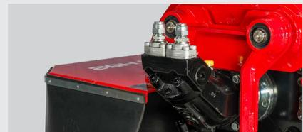
Heavy-duty piston motors simplify construction and remove the need for V-belts.
