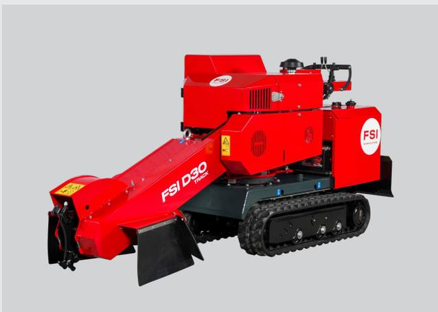
Equipped with counter-rotating tracks, FSI D30 TRACK offers enhanced manoeuvrability and superior traction across a range of terrains. The retractable tracks, combined with the swing-out operator panel similar to the wheeled version, enable the machine to pass through narrow garden gates without compromising the overview of the work area.
