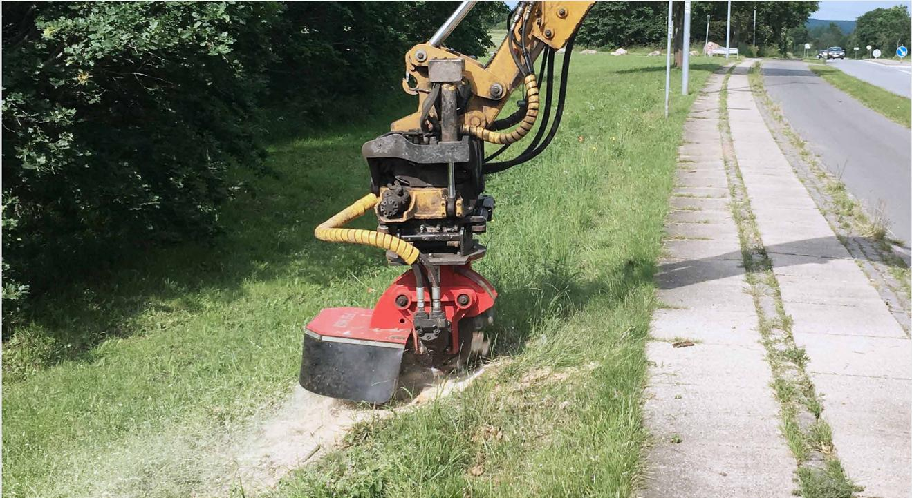
Increase your excavator's functionality by adding a hydraulic-powered stump cutter attachment, ideal for hard-to-reach areas such as slopes, riverbanks, or behind fences and stone walls. Our range accommodates excavators from 2-20 tonnes (15-160 hp).
