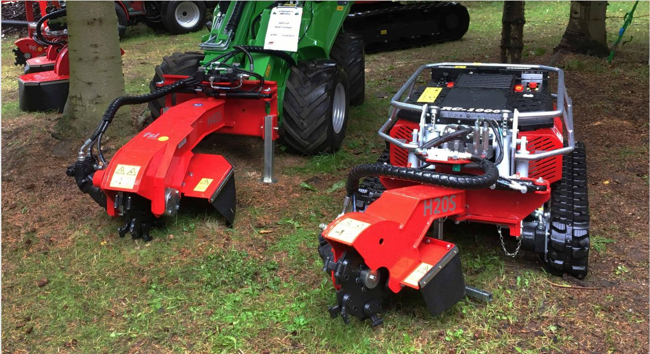
Maximise the versatility of your loader or tool carrier by adding a stump cutter as a tool, allowing stump removal in hard-to-reach areas. Two hydraulic cylinders and an adjustable flow valve ensure a stable sideways sweep controlled either directly from the tool carrier's controls or by an electronic switch box. The stump cutters come with an uncoated back plate, allowing for welding on a suitable attachment. A wide selection of tool attachments is optionally available upon request.
