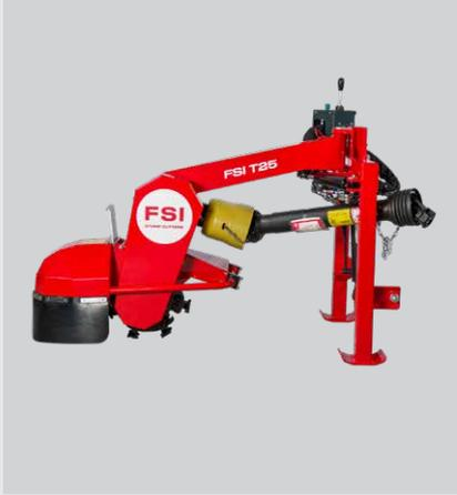
FSI T25 is an economical stump cutter for smaller, category 1 tractors. With a hydraulic toplink that tilts the stump cutter to extend the reach, there is limited need to reposition the tractor during operation.
