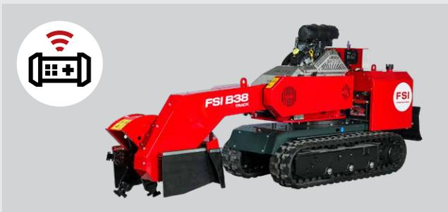
Like FSI B38 4WD REMOTE, the TRACK model is equipped with a remote control system, providing all functions are to hand in stump cutting. A set of counter-rotating tracks offer enhanced manoeuvrability and traction on challenging terrain and can be retracted to allow passage through narrow garden gates.
