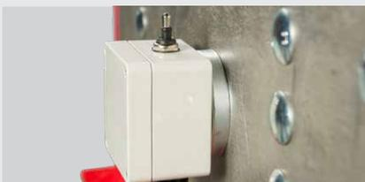
For 3-hose tool carriers, the stump cutter's sweep is operated by an electronic switch, fitted a magnet for convenient positioning near the operator.
