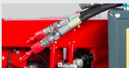
Hydraulic and electrical connectors are included and clearly marked for correct handling
