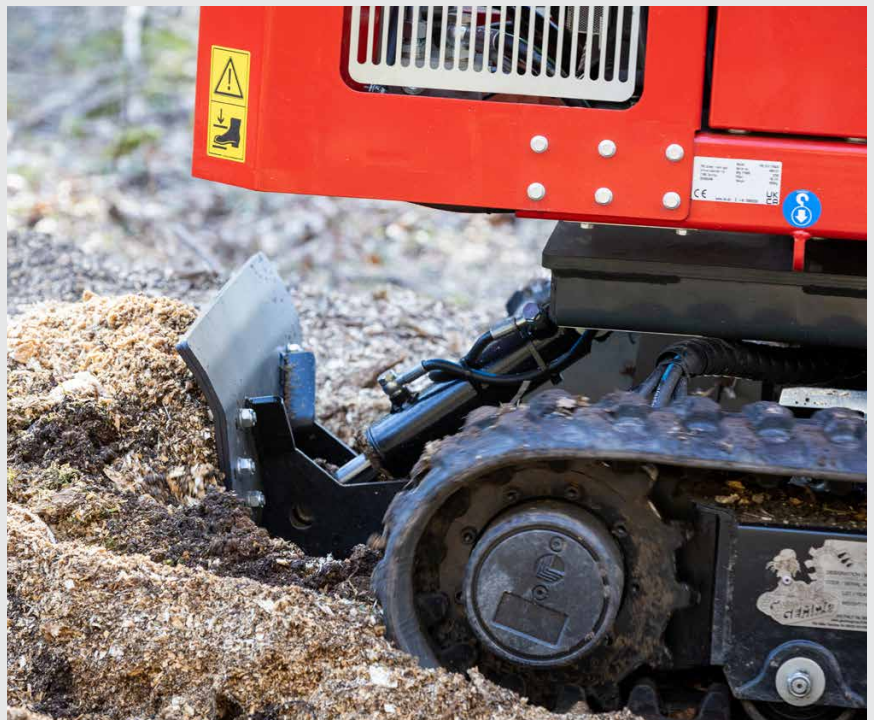
The optional dozer blade eases the process of leveling the ground and refilling after stump removal, leaving a cleaner, more professional-looking work site.
